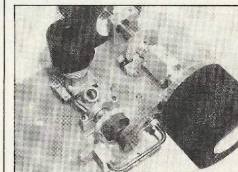
Rear wheel, drive belt and rear axle with differential and pulley drive wheel.
